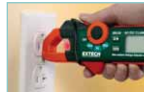
Non-contact voltage detection via clamp tip
