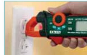
Non-contact voltage detection via clamp tip
